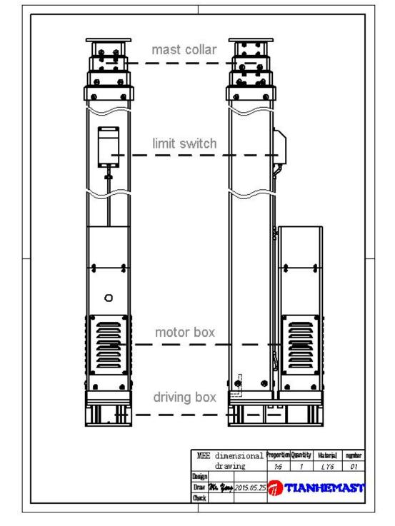
$5.\,4$  Electro screw mechanical mast CAD dimensional drawing.
